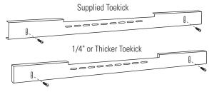
**Important:** The vented toekick must remain unobstructed for proper air circulation and refrigerator operation.
